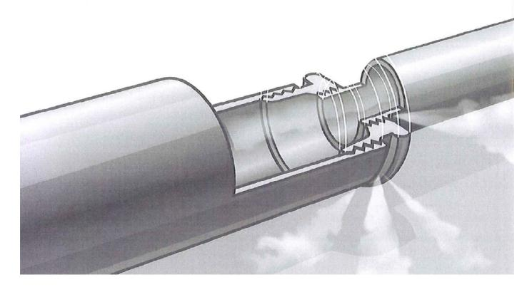
A process for resealing threaded joints of gas pipeworks in buildings
