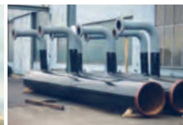
Power plant components: External coating of distribution units
