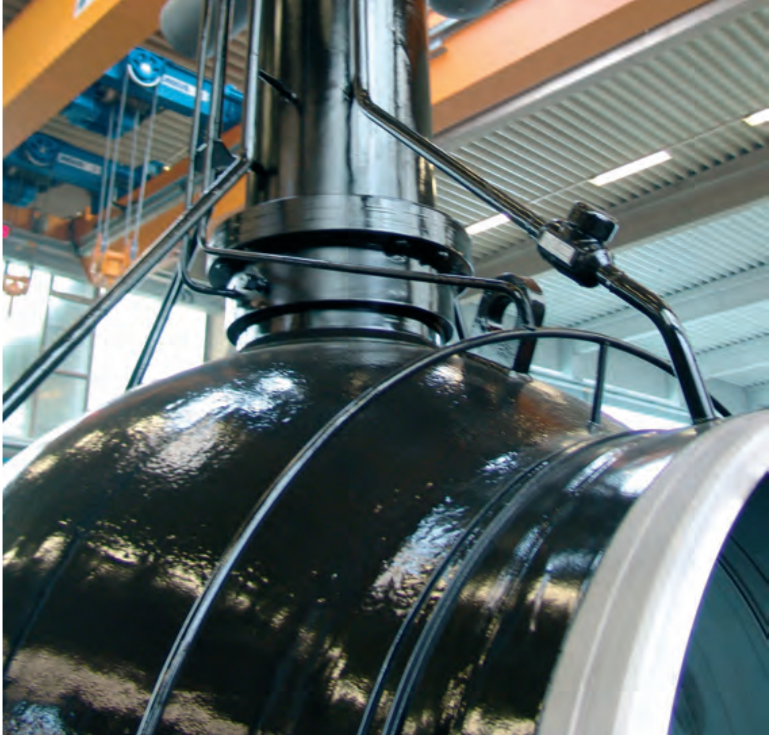
Gas Valves: External coating of 56" ball valve – PROTEGOL®UR Coating 32-55 in a film thickness > 2 mm
